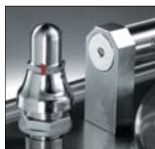
Safety valve for pressure in the jacket
