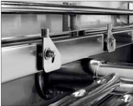
Feeding system fingers are more resistant thanks to their stainless steel construction
