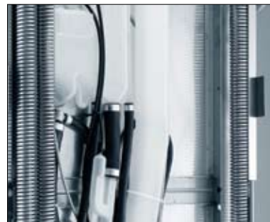
Three springs in the hood lifting system for insulated hood model
